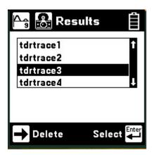
Press the key to select the highlighted result and display the stored results list for that ID number by type (TDR), date and time.
